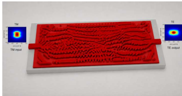
Figure - Topology-optimized TM-to-TE polarization rotator ( 16\ \mu\text{m} \times 6\ \mu\text{m} ) on 4H-SiC-on-insulator.
